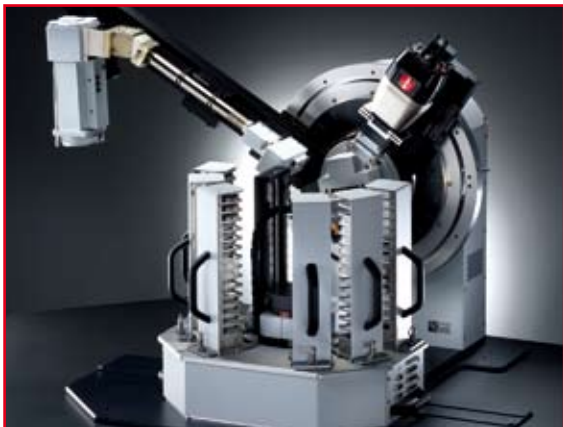
Fig. 3. D8 ADVANCE with Vario1 monochromator in reflection mode, Auto Changer and VANTEC-1 detector.
